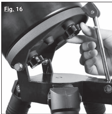
Mounting the MCX on the tilting plate of the tripod.
