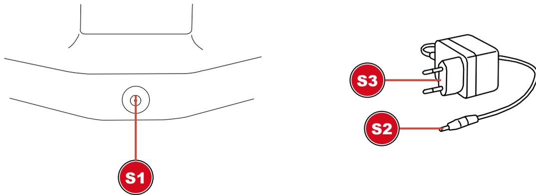
S1 Connection socket for DC barrel connector
