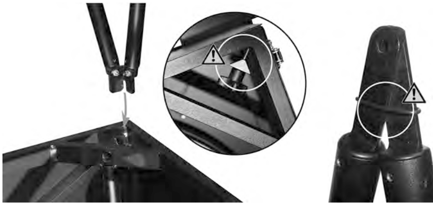
Illustration 3: Mounting the tube trusses
