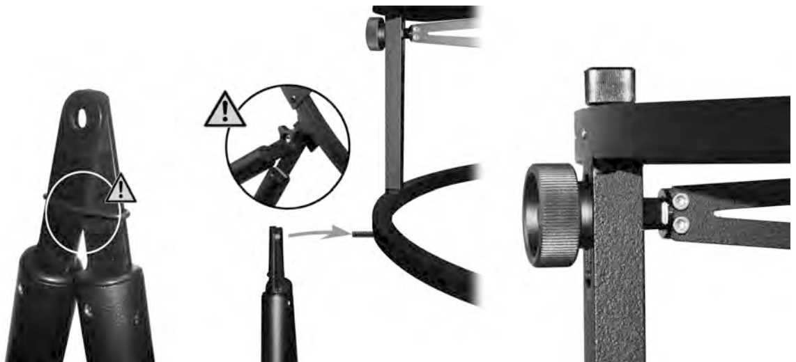
Illustration 5: Mounting the trusses (left) and adjusting screws (right) on the secondary mirror cage.
